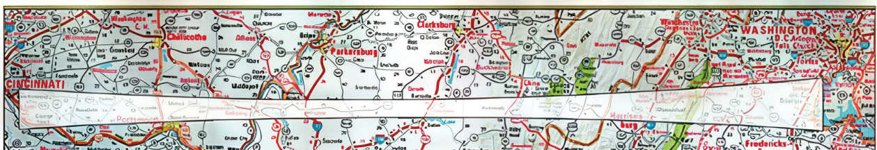
Representation of 370-mile ground scan in a single HEXAGON frame – polar orbit.
